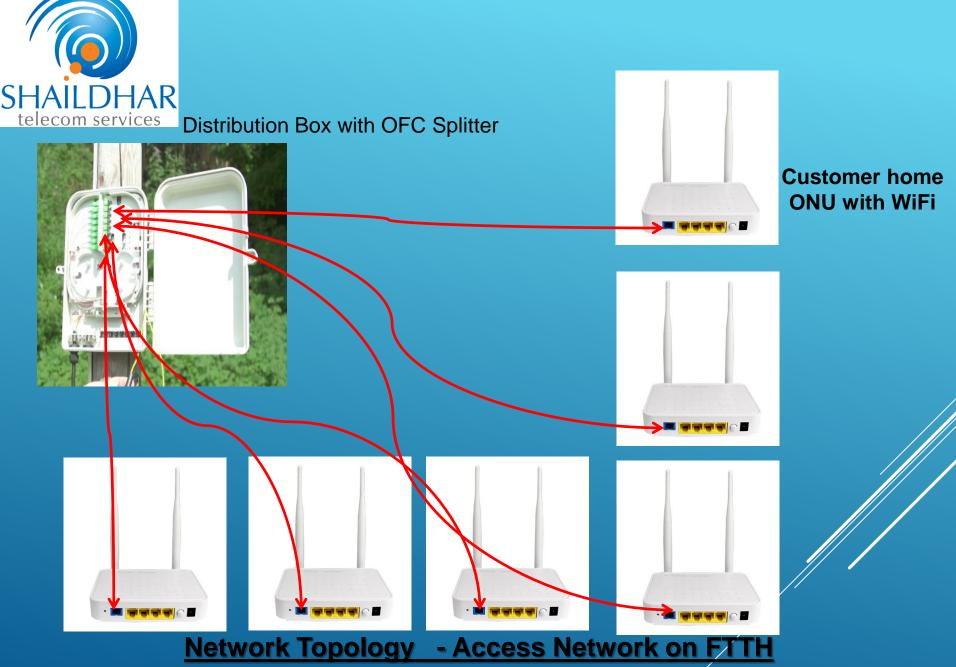
Customer connectivity from Roadside Distribution Box using OFC drop Wires
